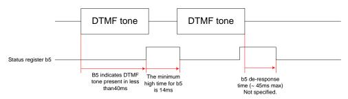
DTMF tones are received under ideal conditions. They are just long enough to be decoded. With good signal conditions, the de-response time is short. B5 is guaranteed to be at least 14ms long so that it cannot be missed due to long polling delays or long interrupt service latency.
