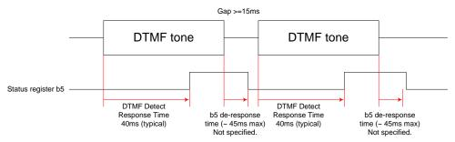
Normal DTMF tones are received and the tone gap is equal to or greater than 15ms (min)
