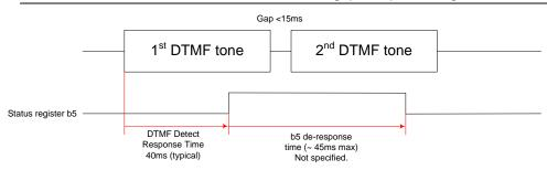
Normal DTMF tones are received but the tone gap is less than 15ms. In this case b5 remains high, there will be no interrupt for the second tone and the DTMF decoder may not indicate the 2<sup>nd</sup> tone value.
