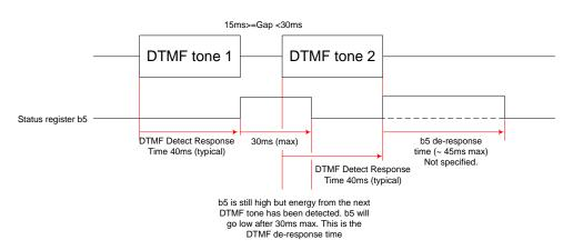
Short DTMF tones (>25ms) are received and the tone gap is less than 30ms but valid. The DTMF decoder will not de-respond in time to re-respond to DTMF tone 2. b5 will not de-assert and signal the new DTMF thus no interrupt can be generated. To avoid this, energy detected after ~15ms will cause b5 to deassert after after 30ms maximum. This is the DTMF decoder de-response time specified. Ie the time that a DTMF tone will be signalled for when DTMF tones have short gaps.
